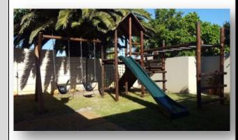
Choose between tapered and cylindrical pine poles. Although both options are equally matched in strength and durability, cylindrical poles have an equal diameter throughout their length giving a neat, clean cut look to your jungle gym. The diameter of tapered poles varies from thick to thin throughout their length and gives a slight rustic look to your jungle gym.
